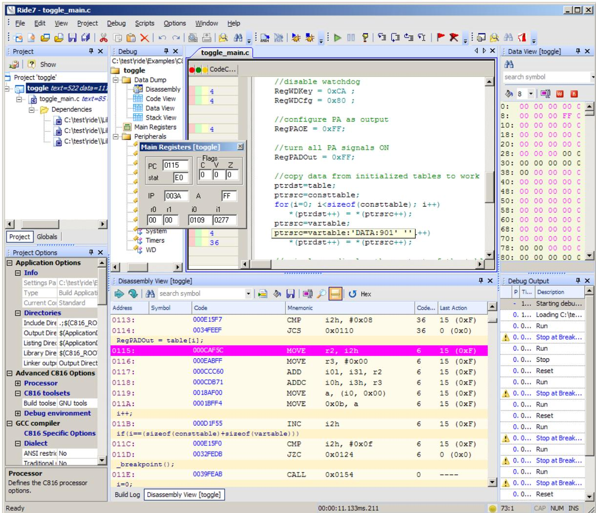
**Note:** From a user interface point of view, basic debugging functions are identical (stopping and resuming CPU execution, setting a breakpoint, single-stepping, checking memory and registers, etc.), whether you are using the simulator or a hardware debug tool. Refer to the Getting Started with Ride7 to get familiar with the simulator before starting to work with the hardware debuggers.
