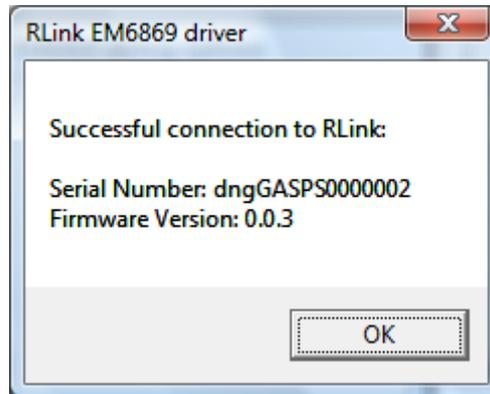
**Note:** This Serial Number is NOT written on the RLink. The only way to find it is with this test.
