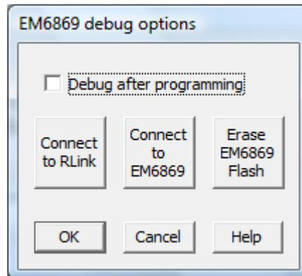
During application development it is sometimes preferable, instead of debugging, to simply program the Flash and let the application run. To do this, terminate the debug session. Go back to the advanced debug options and uncheck the **Debug after programming** checkbox.
